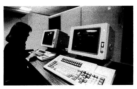
The IBM 3090 Model 200E dual processor, shown here, and the other 3090 models feature Emitter Coupled Logic and Thermal Conduction Modules, and achieve a cycle time of 17.75 nanoseconds.
