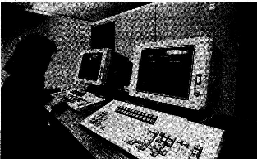
*The newest IBM 3090 S models feature up to 512 megabytes of main memory, up to 2 gigabytes of Expanded Storage, and up to 128 channels.*
