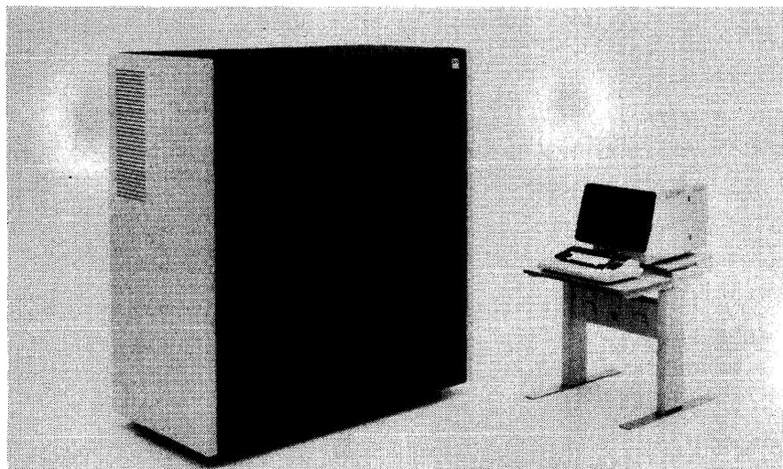
*The 4381 processor features 4 to 16 megabytes of main memory and 32K bytes of buffer storage. The 4381 can support up to 12 I/O channels, and can use virtually all System/370 communications and peripheral equipment. The 4381 supports the MVS/XA operating system, as well as OS/VSI and DOS/VSE.*
