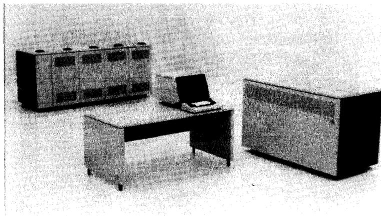
*IBM's 4361 processor systems comprise Model Groups 3, 4, and 5. The 4361 systems are targeted toward department-level computing functions in engineering/scientific and technical environments. The 4361 systems can support up to 12MB of main memory, 241GB of online disk storage, and over 1,000 workstations. The three 4361 models run in IBM's proprietary DOS/VSE, SSX/VSE, and VM operating environments.*
