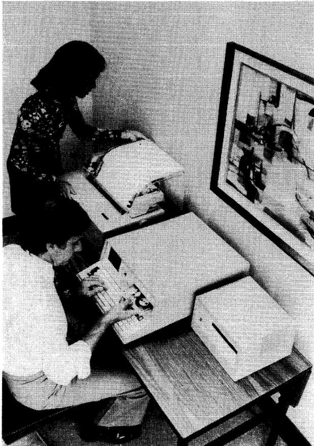
Pictured here is a full-blown 5100 with the optional 80-cps printer and second magnetic tape cartridge unit. The price of this configuration could be as high as \$25,250.
