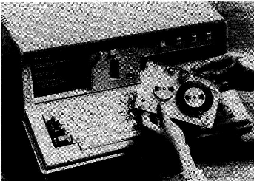
*The 3M-style magnetic tape cartridge is featured in this photo of a basic 5100. The cartridge can store up to 204,000 bytes of data or programs. The built-in CRT can display up to 1024 characters; the characters are rather small, but legible at normal working distances. This 5100 is one of the C series models, which give users a choice between the BASIC and APL programming languages.*
