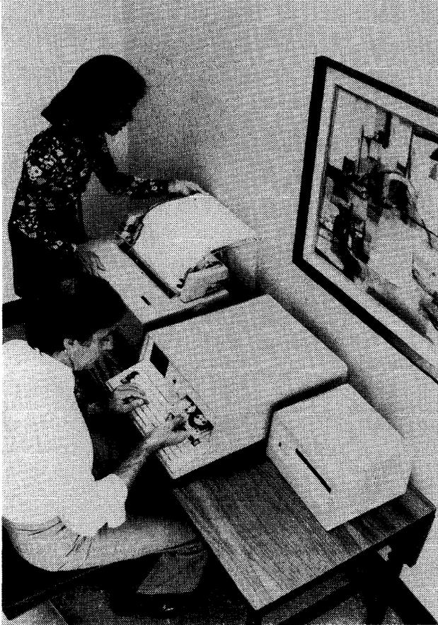
Pictured here is a full-blown 5100 with the optional 80-cps printer and second magnetic tape cartridge unit.
