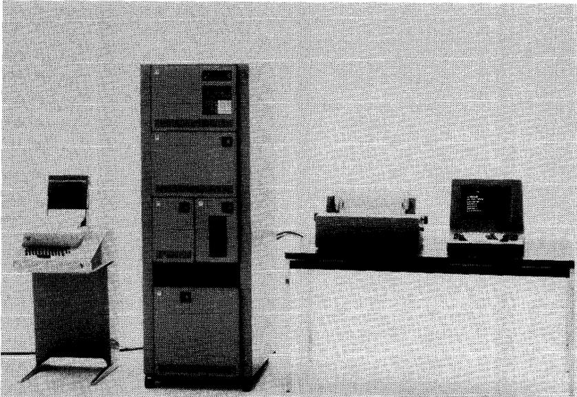
This Series/1 configuration includes a 4997 rack enclosure with a 4955 processor mounted at the top and a 4959 input/output expansion unit below. The bottom half of the enclosure houses a 4962 disk storage unit, with a 4982 sensor I/O unit above and to the left, and a 4964 diskette unit to the right of the sensor unit. Also shown are the 4974 printer, 4979 display station, and a teletypewriter.
