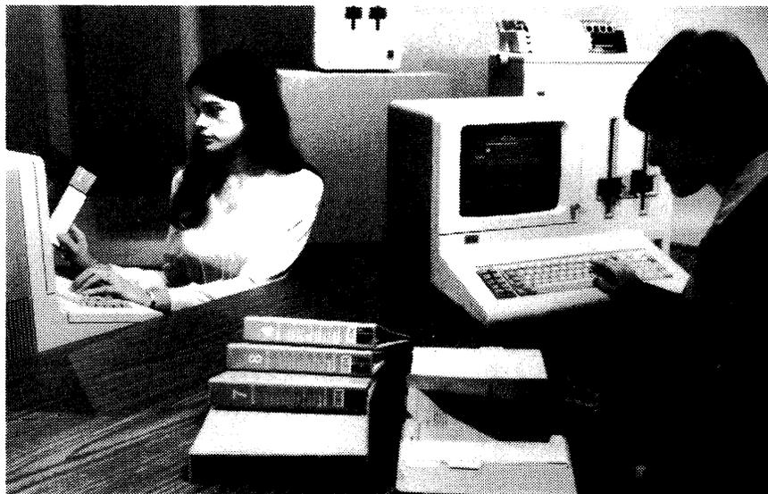
Datamaster, IBM's newest low-cost small business computer system, features an optional dual CPU, workstation configuration which utilizes a separate 2.2-megabyte diskette unit for file sharing. Each computer workstation provides up to 128K bytes of main memory and up to 4.4 megabytes of on-line diskette storage.
