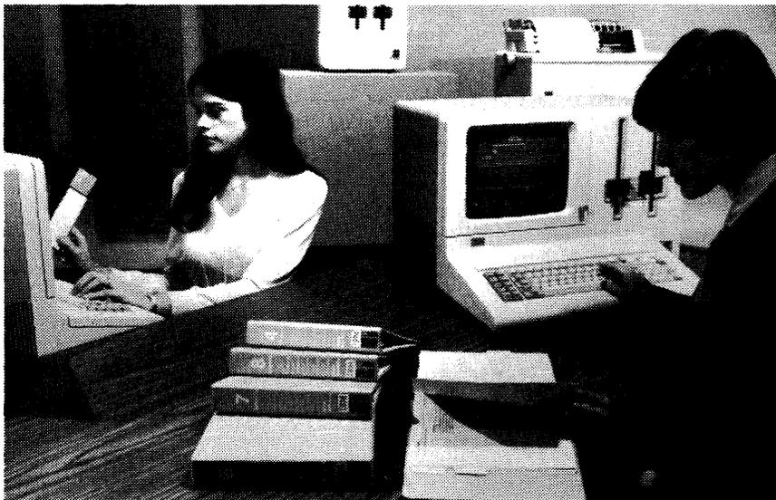
The System/23 Datamaster is a desktop computer designed for first-time users. It features a four workstation/shared file architecture and a functionally enhanced Basic language that is highly compatible with System/34 Basic. A full function data processing and word processing installation with one workstation with 64K bytes of main memory, and an 80 cps printer is priced at \$7,585.
