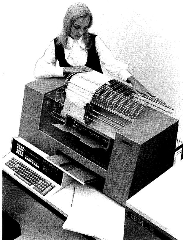
*The wide-carriage 2222 Printer equips this System/3 Model 6 for ledger card processing. As such it competes directly with the small accounting machine variety of business minicomputers.*
