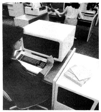
The 5288 Programmable Control Unit (right foreground) provides the processing, control, and storage functions for larger 5280 configurations such as this one. Two keyboard/display stations and a serial matrix printer are also visible in the photo. In a smaller 5280 configuration, the processor, 32K to 64K bytes of main storage, and one or two diskette drives are all housed within one of the table-top keyboard/display stations.
