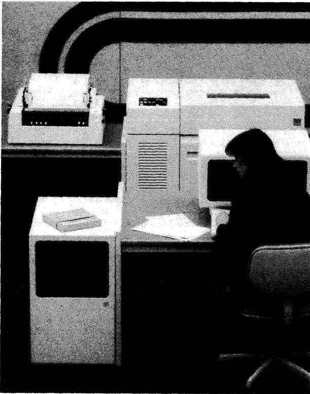
*The 5288 Programmable Control Unit (bottom left) provides the processing, control, and storage functions for larger 5280 configurations such as shown above. Also included in this configuration (clockwise) is a 5256 bidirectional serial matrix printer, a 5225 wire-matrix line printer, and a 5281 Data Station.*
