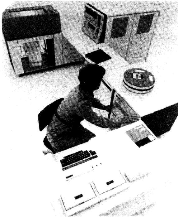
*IBM's first totally cardless System/3 is the new Model 8. It is designed for batch processing and convenient addition of communications, thanks to the first Integrated Communications Adapter available on a System/3. In the foreground, the operator is seated at a directly attached 3741 Data Station, whose interchangeable diskettes substitute for card I/O. A typical system as shown rents for about \$1,849 or sells for \$72,075.*
