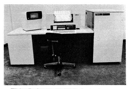
The last model announced in the System/3 product line was the Model 4, introduced in January 1976. The Model 4 is designed to handle multiple workstations, including IBM 3277 CRT Displays, 40-cps 3284 Serial Printers, 66-cps 3286 Serial Printers, and 120-cps 3287 Serial Printers, and 120-lpm 3288 Line Printers. A basic Model 4 configuration can be purchased for \$36,357.
