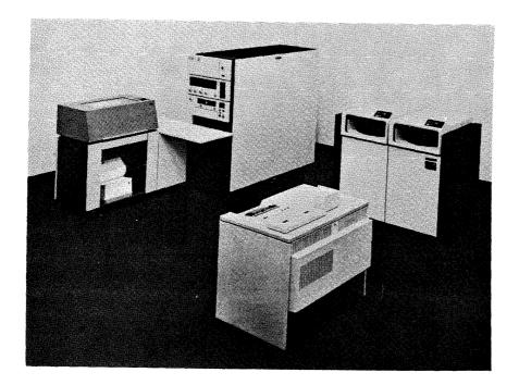
The System/3 Model 12, like the Models 4, 6, 8, and 10, has a memory cycle time of 1.52 microseconds and an add time for 5 digits of 24.32 microseconds. The Model 12 is available in 12 submodels varying in main memory capacity from 32,768 bytes to 98,304 bytes and has a disk storage capacity of up to 82 megabytes. A basic Model 12 system is priced at \$100.331.
