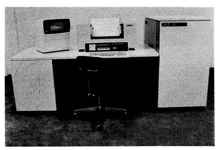
The last model announced in the System/3 product line was the Model 4, introduced in January 1976. The Model 4 is designed to handle multiple workstations, including IBM 3277 CRT Displays, 40-cps 3284 Serial Printers, 66-cps 3286 Serial Printers, 80- and 120-cps 3287 Serial Printers, and 120-lpm 3288 Line Printers. A basic Model 4 configuration can be purchased for \$36,357.
