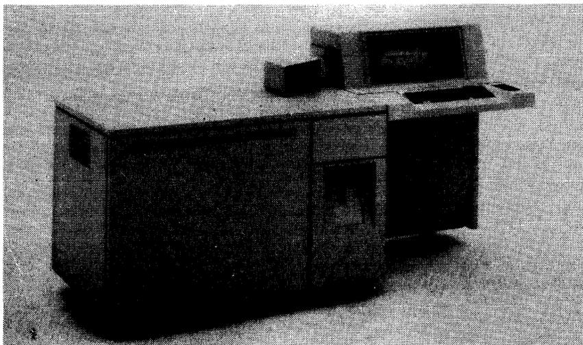
IBM's highly successful small business computer, the System/32, is a compact, desk-sized system available in 32 different models. Each model has either a serial or line printer, available in several speeds, and four different levels of fixed disk capacity. Using IBM's Industry Application Programs, the System/32 is an ideal system for first-time computer users.
