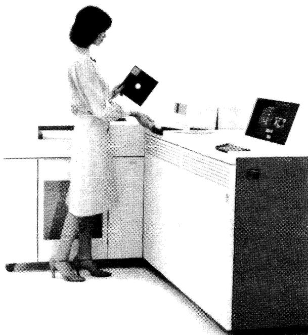
One of the more important units that is integral to the 5381 System Unit is the diskette magazine drive. This unit provides three functions; save/restore, diskette I/O, and CE servicing. The storage capacity of each diskette depends on type and formatting. Three types of diskette may be read by the unit in three different formats. Maximum capacity for the drive is 24 million bytes.
