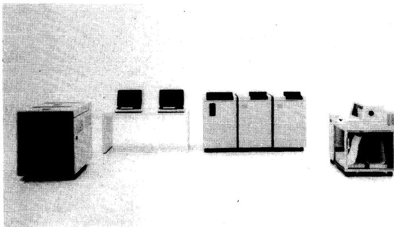
This IBM 8100 configuration includes, from left to right: two 8809 Magnetic Tape Units, two 8775 Display Terminals, an 8100 Processor, two 8101 Storage and I/O units, and a 3289 Line Printer, Model 3. An 8100 system can support up to 1024K bytes of memory and 639 megabytes of disk storage.
