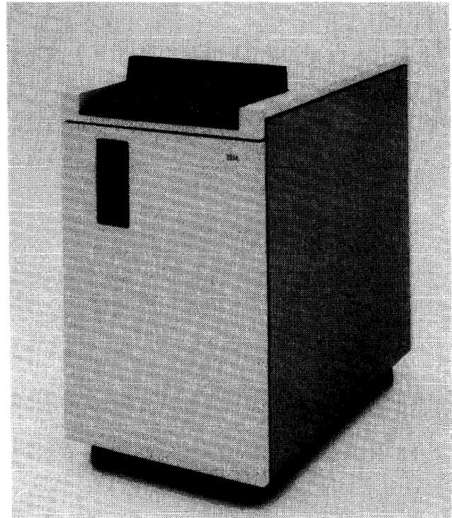
The 8140 processor is shown with the Expanded Function Operator Panel (EFOP). Supplied in addition to the basic panel as a program diagnostic aid, the EFOP provides programmer and operator access to storage, program stop and restart capability, and current operating indicators.
