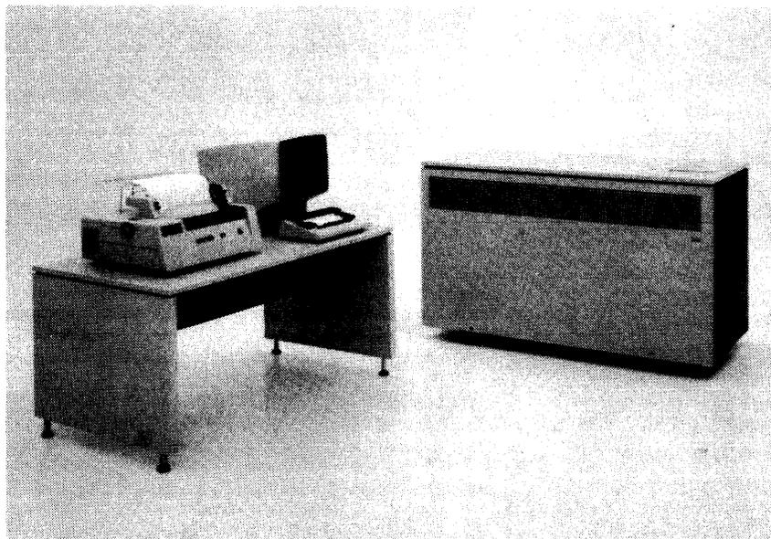
The smaller processor in IBM's new series, the 4331, can fit easily into an office environment. Shown here are the processor complete with its integrated adapters (right) and the system console with a hard-copy device. Missing from the photo are the two other elements needed for a basic 4331 configuration: a line printer and the new 3310 Direct Access Storage Device.
