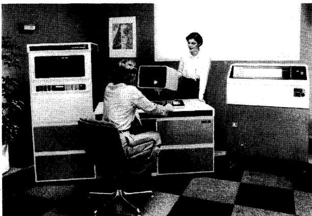
*The ME29 range of medium-scale workstation-oriented systems offers extensive communications facilities. On the left is the processor and either one or two floppy disk drives. A multipurpose workstation is on the control desk, which also houses two 35MB fixed disk drives. On the right is a 600 lpm line printer.*
