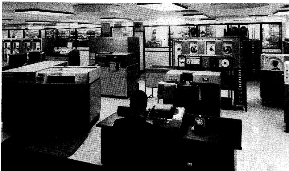
*The small-scale 1901A system is spotlighted in this view of ICL's program testing installation in London. At left is the central processor cabinet, which also houses the line printer. Ranked behind the operator's console are a card reader, paper tape reader/punch, and four magnetic tape drives. At far right are two Twin Exchangeable Disc Store (TEDS) units.*
