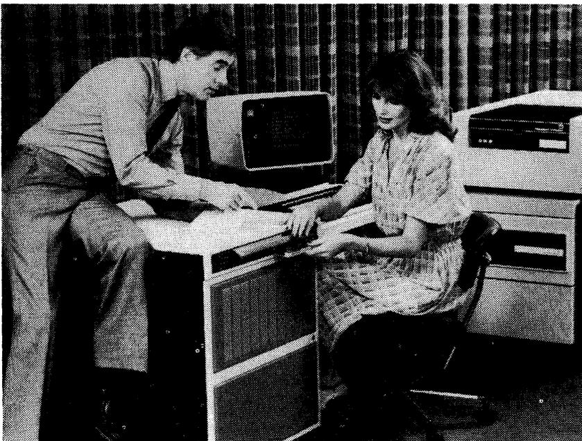
ICL's new System 25 includes a cabinet that contains processors, memory, a Winchester disc drive, and tape cartridge drives for software exchange. Also shown is a Model 85 visual display unit, one of several workstations available, and, at right, a fixed and exchangeable disc file.
