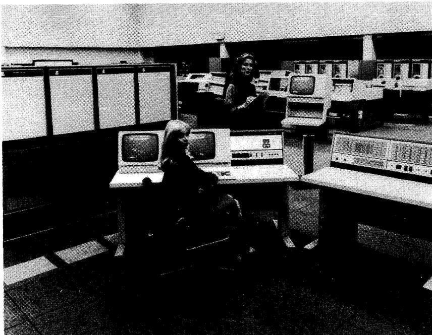
*This ICL 2970, one of four medium to large scale 2900 Series systems currently available, includes a dual-screen Master Operating Station and, at right, a reconfiguration console. Remote monitors, such as the one behind the consoles, enable operators to receive system messages and alarms while they are away from the master console.*
