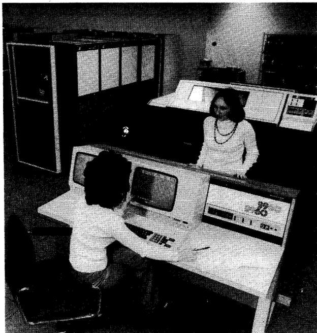
*This ICL 2960 system includes a dual-screen master console, an LP-1500 line printer, and, in the four-bay cabinet, a central processor with 524,288 bytes of memory. The left console screen displays system status; the right screen displays the most recent operator commands and the system's responses. An engineer's control processor, built into the end of the central processor cabinet, includes a keyboard, a display, and a cassette reader.*
