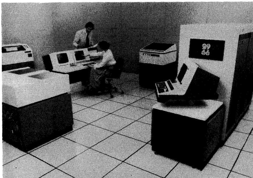
One of the most recently announced models, the ICL 2966 falls in the middle of the range between the 2946 and the 2982. The system shown is equipped to run in the Concurrent Machine Environments mode and has both a 2966 console, foreground, and a George 3 console, background, for controlling 1900 series emulation.
