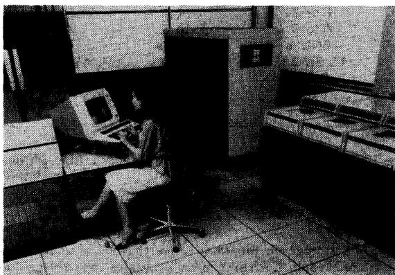
*Picture shows the ICL 2966 mainframe computer which can be configured with single or dual processors having up to 32M bytes of store.*
