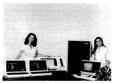
The top-of-the-line Reality Series 8000 was introduced in October 1979 and includes two models, the 8750 and 8770. The basic 8750 configuration includes 256K bytes of MOS memory and 128 million bytes of disk storage. A basic 8770 system includes 256K bytes of MOS memory and 256 million bytes of disk storage. Both models are expandable to up to 514 million bytes of disk storage and up to 32 CRT terminals.
