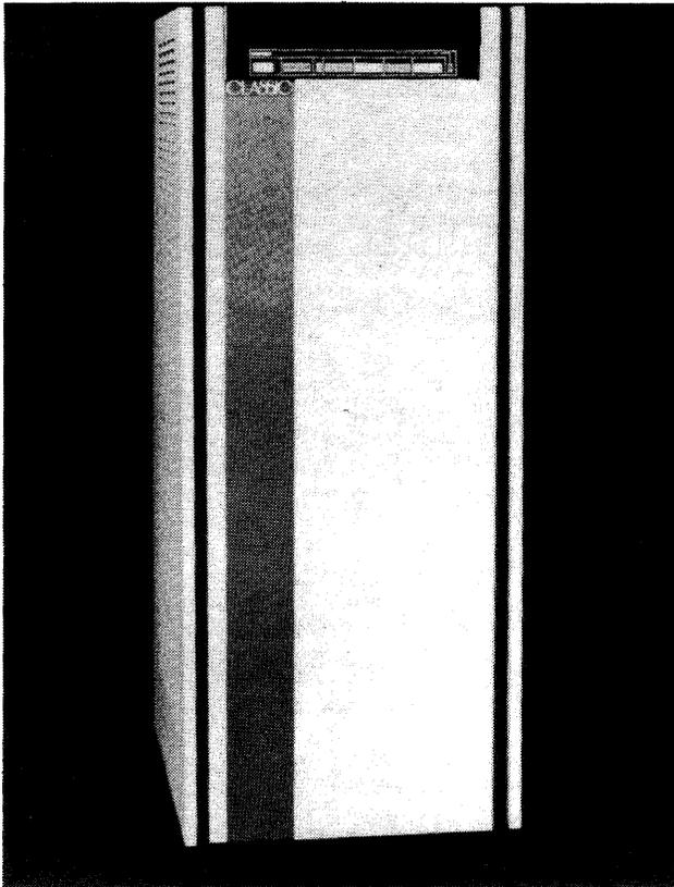
The Classic 7810 is designed for use in lower level measurement and control, scientific, and information processing applications. The 7810 is available either as a computer-on-a-board or as a fully integrated system. Features include a set of 169 instructions, 15 general purpose registers, and system protect. The 7810 is available in three versions with 64K, 96K, or 128K bytes of solid state memory that has an effective cycle time of 600 nanoseconds.
