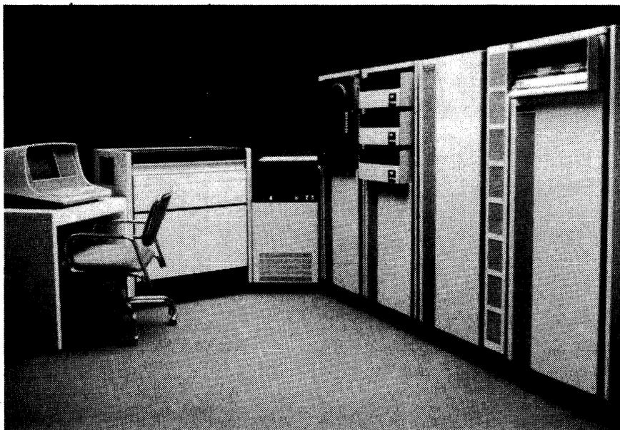
Modcomp's Classic 7870 features memory capacity of up to two million bytes. A Shared Multiport Memory system (SMM) extends this capacity to four million bytes as well as allowing users to configure shared memory systems. Both the 7860 and 7870 models include an integral high-speed floating-point processor that performs operation in 32-, 48- or 64-bit operands in parallel. As a standard feature, the 7860 and 7870 systems have five concurrent memory access paths.
