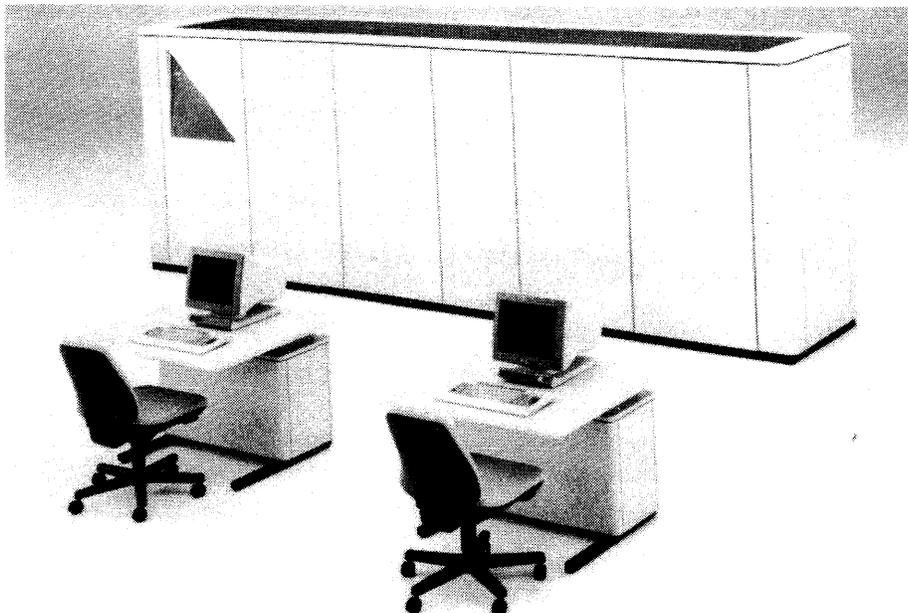
The top-of-the-line AS/XL Series is available in a single- or a dual-processor model that is comparable in performance to IBM's 3090 Series. The AS/XL processors have from 64 to 256 megabytes of main memory and from 16 to 64 I/O channels. The system features VLSI circuits throughout, and a one-megabyte dynamic working storage caching system between the main memory and the cache buffer.
