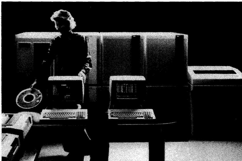
*The NCR 9800 is an on-line transaction processing system, based on multiple function-specific processors. The 9842 model is a mid-range configuration consisting of four Application Processors and two Data Storage Processors. Each Application Processor can contain up to 8 megabytes of memory and each Data Storage Processor has a memory capacity of 16 megabytes.*
