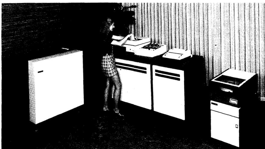
*One of the two May 1974 additions to the NCR Century Series computer family, the compact Century 151 is the first to utilize MOS main memory. The Basic System pictured here features 32K bytes of 750-nanosecond MOS memory, an integrated 300-lpm line printer and 300-cpm card reader, and 9.8 million bytes of disc storage.*
