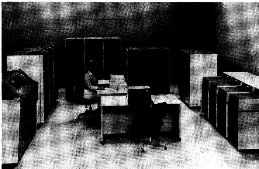
*NCR's V-8500 Group II Series includes seven models that can have from one to four CPUs, one to eight megabytes of memory, and a wide range of I/O devices. Performance is comparable to the IBM 4300 Series.*
