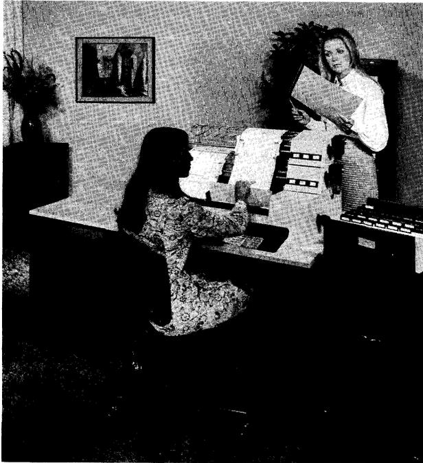
*The NCR 399 can be equipped to read high-density magnetic-stripe ledger cards and to feed two continuous forms under independent program control.*
