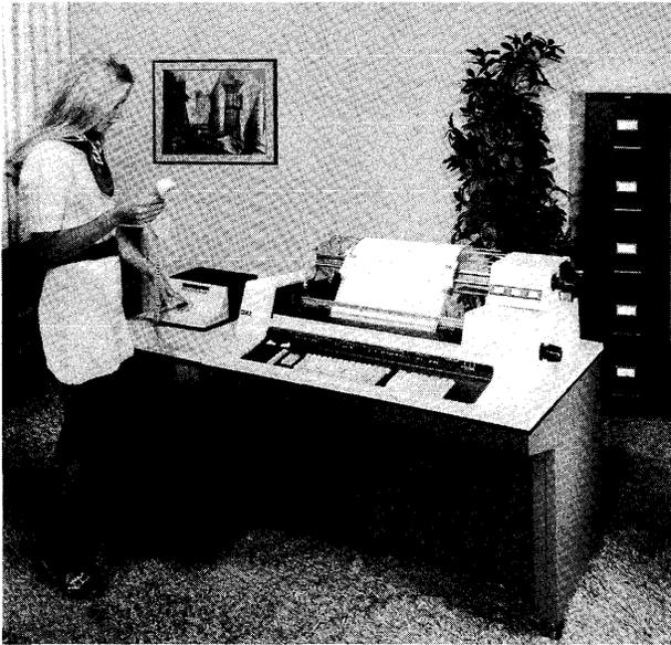
*When equipped with a synchronous or asynchronous communications adapter, the NCR 399 serves as an intelligent terminal that can handle editing, formatting, validating, and batching of input data for transmission to a remote computer.*
