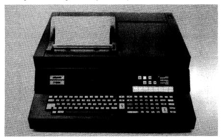
The desktop P6060 includes a 32-character visible display, an 80-column, 80-cps thermal matrix printer with plotting capabilities, a full ASCII alphanumeric keyboard with BASIC verbs, a floppy disk unit, and an operating console and lights. The basic unit can be supplied with one or two peripheral interfaces, each allowing up to four 1/O units to be connected. A moving-head disk unit can also be added.
