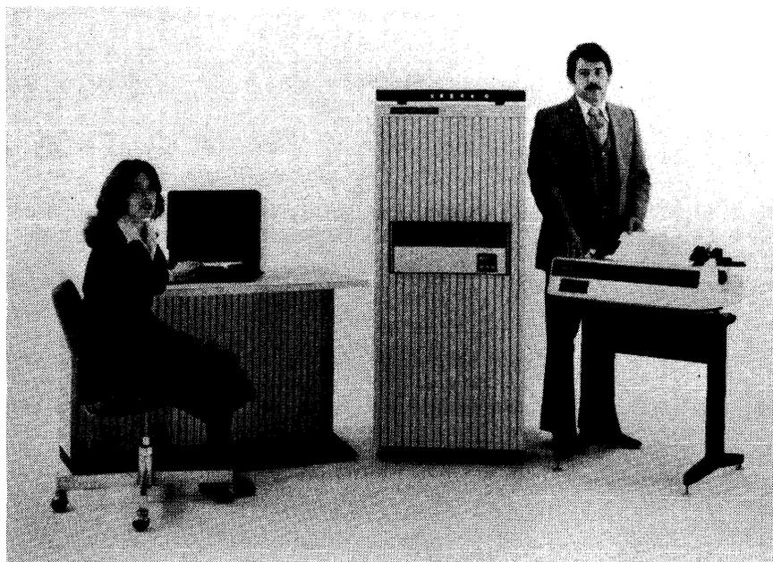
*The top of the Series Sixteen line is the 1635, based on a 16-slot CPU. The Error Checking and Correcting MOS memory is field-expandable from 128K to 256K bytes on a single memory board. The 1635 supports single- and single/double-precision floating-point processors and has hardware multiply/divide, privileged instruction detection, memory processor integrity test, and optional battery backup for two hours.*
