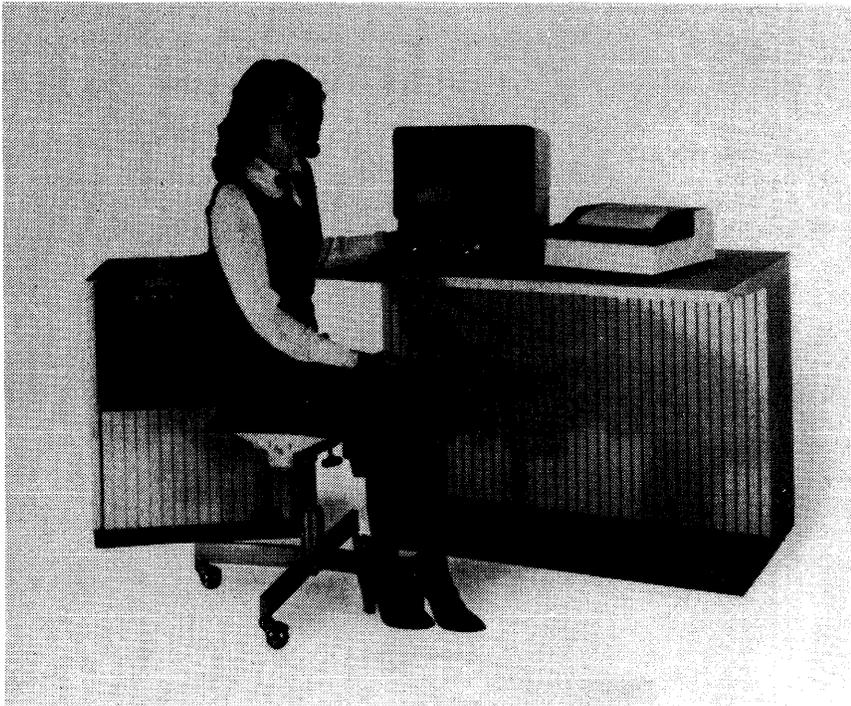
*The 1615 System, low end of Perkin-Elmer's Series Sixteen, has from 32K to 64K bytes of parity MOS memory, multiply/divide and list processing instructions, 255 hardware-vectorized interrupts, and an eight-slot chassis. Available peripherals include a 512K-byte floppy disk drive, a Model 550 video display unit, and a Model 655 thermal page printer.*
