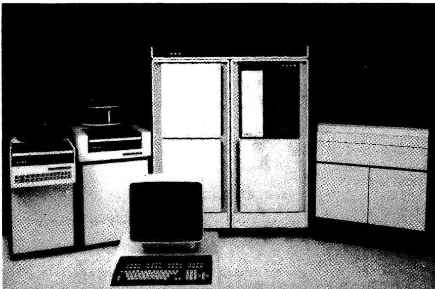
The Series 50 from Prime includes four systems with 32-bit architecture. The photo shows (left to right, rear) 80- and 300-megabyte disk subsystems, the Prime Series 50 CPU (as used in Models 550, 650, and 750) with a magnetic tape subsystem, and the 600-lpm line printer. A block-mode visual display unit is in the foreground. The Series 50 systems support up to 63 simultaneous users, up to 8 million bytes of main memory, and a 32-million-byte virtual address space for each user.
