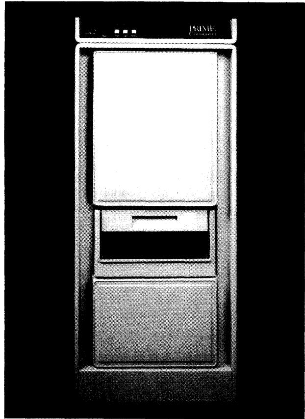
This photo of the Prime 450 CPU shows the five switches and four lighted indicators of the VCP (Virtual Control Panel) at the upper left of the cabinet. The VCP, a standard feature on all Series 50 models, allows the system to be accessed by an authorized local or remote terminal for purposes of system operation or local or remote diagnosis.
