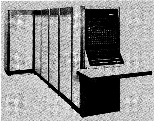
The System 4004/150, Siemens' own adaptation of the former RCA 6 Processor, offers up to 2 million bytes of core storage.
