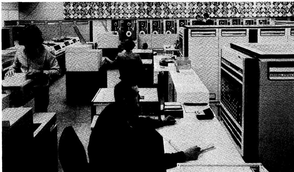
*Siemens' medium-scale System 4004/45-III is based upon the RCA Spectra 70/45 (now the UNIVAC Series 70/45). Two Model 45-III Processors are shown here, along with three card readers, six disc drives, and twelve magnetic tape units.*
