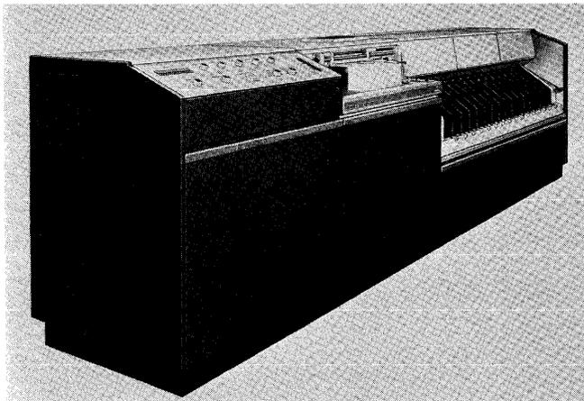
The 4250 Optical Document Reader/Sorter has 16 pockets, can be used either on-line or off-line, and reads characters printed in various fonts, including OCR A, OCR B, and IBM 407.
