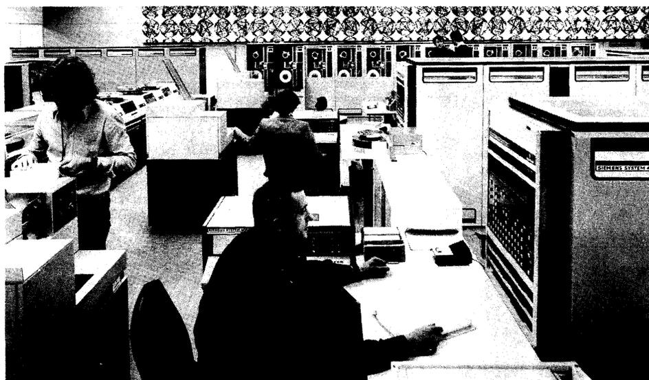
Two Model 45-III Processors are shown here, along with three card readers, six disc drives, and twelve magnetic tape units.
