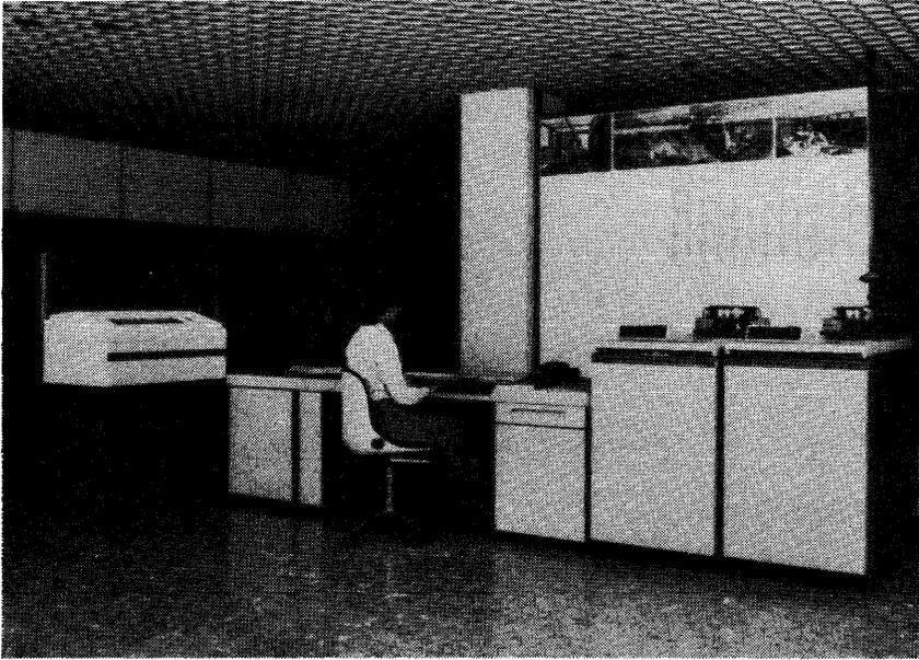
The System 7.521, the entry-level model in the Siemens System 7.500 series, is designed for office environments. The central processor and the central workstation are built into a desk-sized enclosure.
