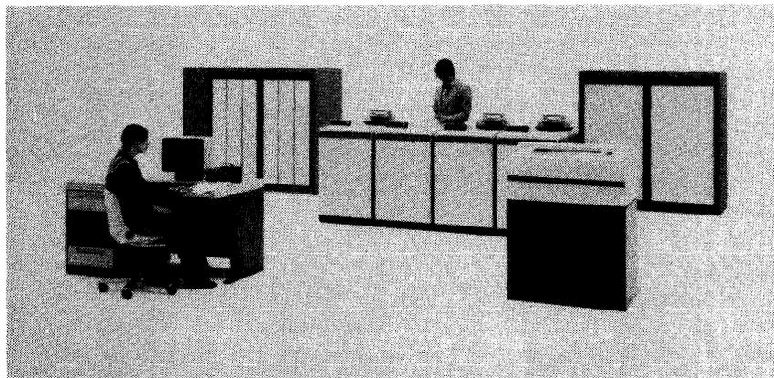
The System 7.541, the largest of the three Siemens System 7.500 models, is designed for climate controlled computer centers. The other, smaller models, the System 7.521 and System 7.531, are designed for office environments. The series is upward compatible with the larger Siemens System 7.700 family.
