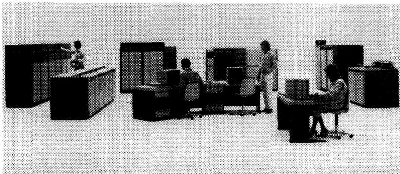
Scheduled for delivery the first quarter of 1982, the System 7.571 is the largest of the seven Siemens 7.500 models, and is approximately as powerful as IBM's 3033 and Siemens' own plug-compatible mainframe 7.872. The basic configuration is composed of the central processing unit, a main memory of four megabytes expandable to eight megabytes, a cache memory of 64K bytes, and one input/output processor with six block multiplexor channels. A theoretical maximum of 384 disk drives can be supported.
