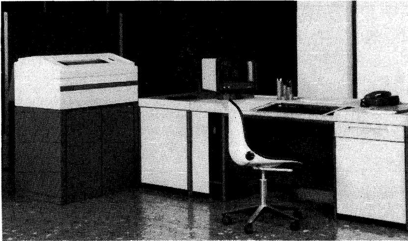
As the 7.500 Series entry-level model, the 7.521 compact computer comes with 512K bytes of main memory and is built into a desk enclosure with system keyboard/display, floppy disk drive, a direct disk storage adapter, and a 300-line-per-minute printer. The 7.521 can be operated by non-technical staff in an office environment.
