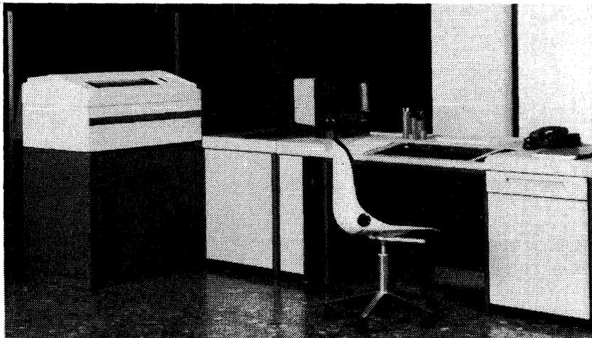
As the 7.500 Series entry-level model, the 7.521 compact computer comes with 512K bytes of main memory and is built into a desk enclosure with system keyboard/display, floppy disk drive, a direct disk storage adapter, and a 300-line-per-minute printer. The 7.521 can be operated by non-technical staff in an office-environment.
