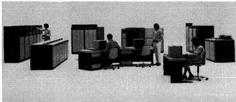
The System 7.571 is the largest of the seven Siemens 7.500 models, and is approximately as powerful as IBM's 3033 and Siemens' own plug-compatible mainframe 7.872. The basic configuration is composed of the central processing unit, a main memory of four megabytes expandable to eight megabytes, a cache memory of 64K bytes, and one input/output processor with six block-multiplexor channels. A theoretical maximum of 384 disk drives can be supported.
