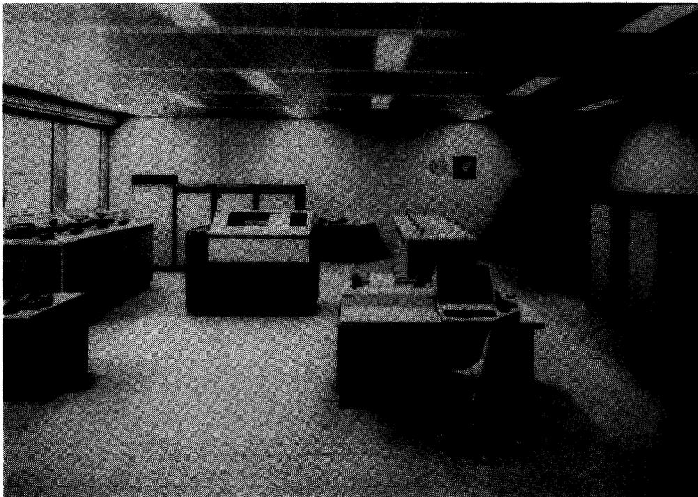
*This 7.760 configuration includes a 2.5 megabyte main memory, a 3020 Central Operator Console with 3033-01 Printer, a 3020-10 Auxiliary Console, four 3460 Disk Drives (200 megabytes each), one 3470 Fixed Disk Drive (420 megabytes), a 3343 Line Printer (1630-2000 lpm), four 3540 Magnetic Tape Drives (1600 bpi, 120 kilobytes per second), and a 9684 Transdata Data Communication unit capable of supporting up to 42 remote terminals.*
