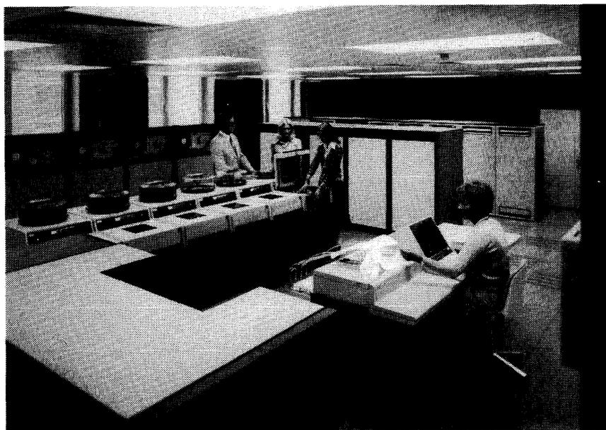
*Each of the Siemens 7.000 models offers a wide variety of operator console configurations. Shown here is a 3030 Central Console with a CRT, keyboard, tabulator, control panel, and a 180-cps hardcopy page printer (Model 3030). Up to three auxiliary consoles (3020-10 or 3023-10) can be located up to 10 kilometers from the CPU and can be attached to any Series 7.000 model.*
