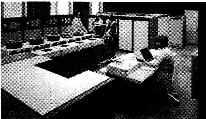
Each of the Siemens 7.700 models offers a wide variety of operator console configurations. Shown here is a 3030 Central Console with a CRT, keyboard, tabulator, control panel, and a 180-cps hardcopy page printer (Model 3030). Up to three auxiliary consoles (3020-10 or 3023-10) can be located up to 10 kilometers from the CPU and can be attached to any Series 7.700 model.
