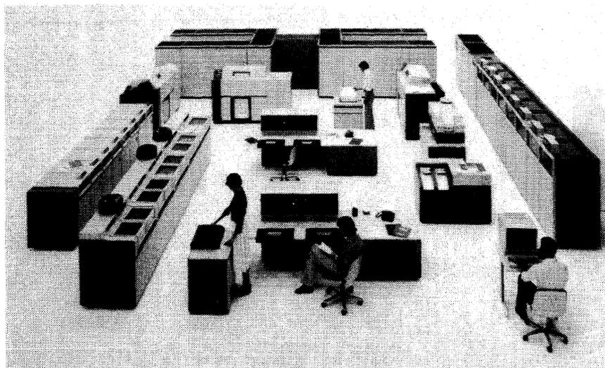
Currently the largest model in the Siemens System 7.800 series, the dual-processor 7.882 is designed as a compatible upgrade for large IBM System 360 and System 370 systems.
