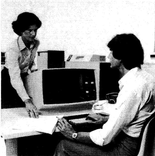
The 3807 console for the 7.870 includes a color display and an integrated cartridge disk drive for loading diagnostic software. Dual-processor 7.872 models require two 3807 consoles.
