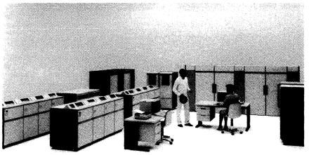
The 7.570-P is the most powerful of the 10 Siemens 7.500 models. It is a dyadic system that contains two CPUs, and two central operator consoles as shown. The main memory range of the -P is 16MB to 64MB.
