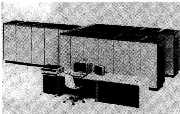
Pictured is the Siemens 7.890. The 7.800 Series compete with the IBM 4300 and 30XX Series. Main memory ranges from 12 to 32 megabytes.
