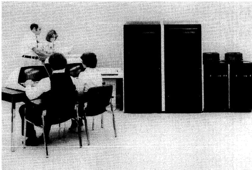
*Tandem Non-Stop Systems can be configured to include up to 16 processor modules with either core or MOS memory and a variety of peripherals. The Guardian/Expand communications network can accommodate up to 255 geographically dispersed systems, each with a maximum of 16 central processors.*
