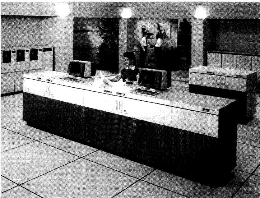
*The Unisys A 10 HX is an intermediate-range, dual-processor mainframe with up to 96 megabytes of main memory, two I/O cabinets with a maximum of 80 DLPs, and up to 288 data communication lines.*
