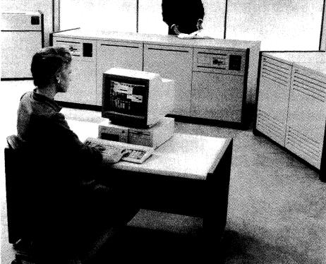
The Unisys 2200/200 Series has from one to four central processors, 32K bytes of cache memory per processor, and a main memory capacity ranging from 8 to 48 megabytes. Up to eight integrated disk drives can be added to the basic 2200/200 cabinet, which occupies only 10.5 square feet of floor space and plugs into a standard 220-volt outlet.
