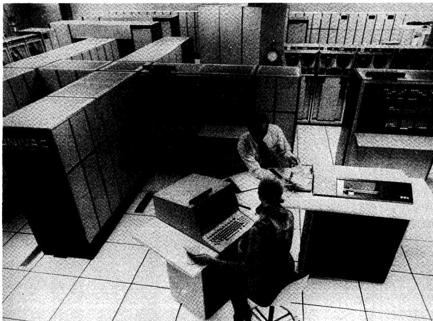
UNIVAC's large-scale 1106, 1108, and 1110 systems combine powerful hardware facilities with advanced software to achieve impressive performance levels. The top-of-the-line 1110 system features multiple processors, two levels of directly addressable storage, and independent I/O controllers and communications processors.
